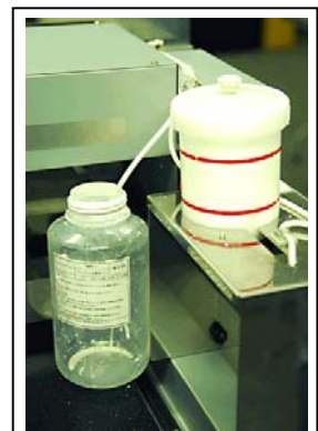
Figure 1: Empty the white ink into an appropriate storage bottle.
